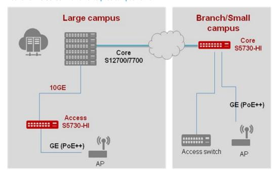
Huawei S5730-HI is the next-generation fixed agile switch. The S5730-HI has large table sizes and buffers, avoiding packet loss in traffic bursts. It supports wired and wireless convergence and unified management on devices, users, and services. The S5730-HI can be used as the core device on an enterprise branch network or a small campus network or as the aggregation or access device on a large campus network, to achieve a manageable and reliable enterprise campus network with scalable services.
